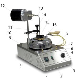
1. Main Power Switch. Controls power to the entire unit. Pressing the switch to the ON position will energize the instrument. Pressing the switch to the OFF position will de-energize the instrument. Switch will illuminate when in the ON position
