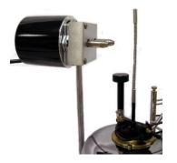
After approximately 100 hours of use, remove the motor cover and locate the two drive shafts. Place a few drops of light lubricating oil such as **3 in 1** into the bottom of each shaft and re-install the motor cover.
